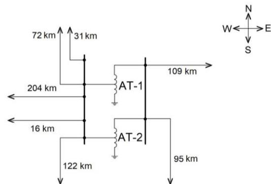
Figure 2. System diagram of the Vykhodnoy 330 kV substation
