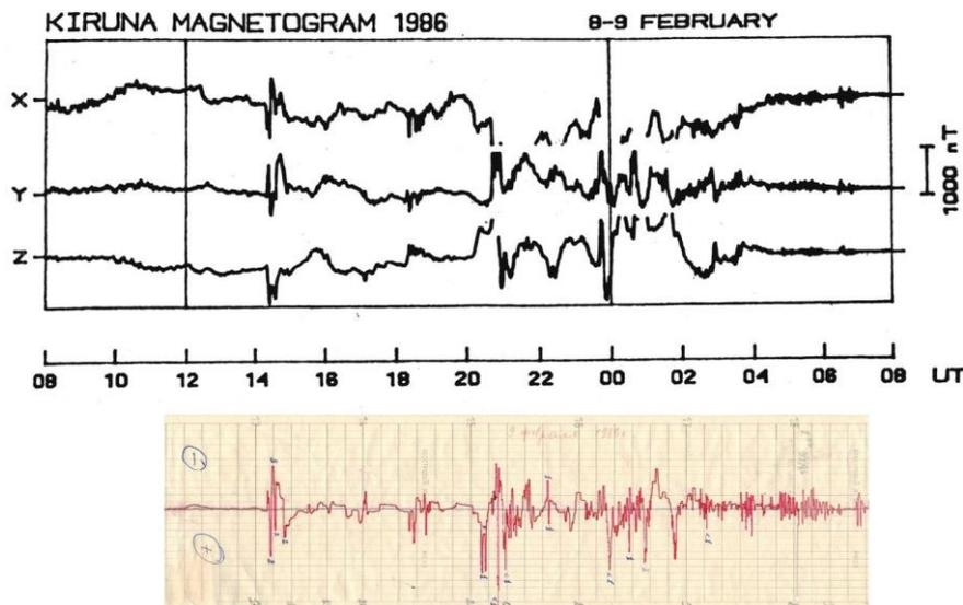
Figure 3. Time coincident oscillograms of GIC in a transformer neutral and magnetograms of geomagnetic variations
