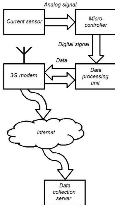
Figure 4. Schematic diagram of a GIC recorder
