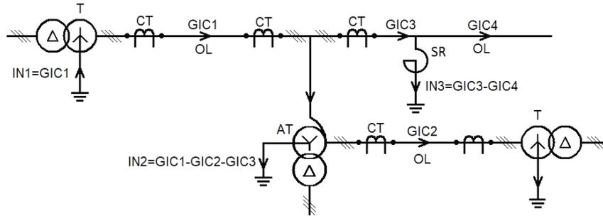
Figure 1. Geomagnetically induced currents in a branched electrical grid: T — transformer, AT — autotransformer, CT — current transformer, SR — shunt reactor, OL — overhead transmission line, GIC — geomagnetically induced current, IN — current in a grounded neutral
