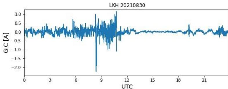
Figure 9. GIC variation in the transformer neutral as the electrical grid topology changes
