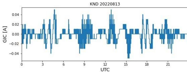
Figure 8. Neutral current in a disconnected transformer
