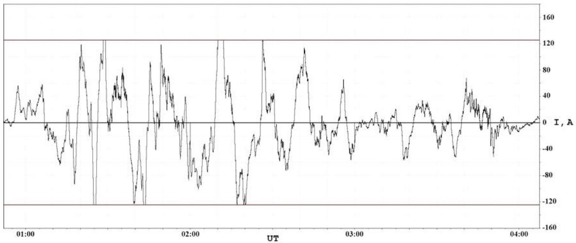
Figure 7. Signal clipping (June 29, 2013)
