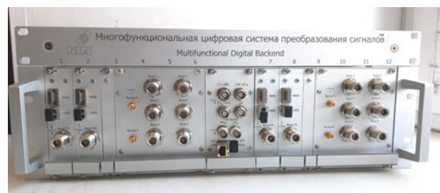
Figure 2. Four-channel MDBE system for radio telescopes RT-32
