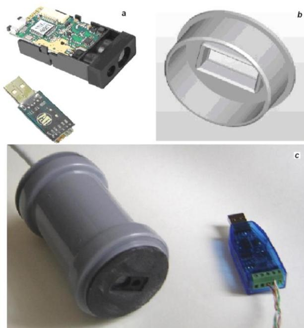
Figure 5. Laser rangefinder module (a); case cover into which the module is inserted (b); rangefinder assembly (c)
