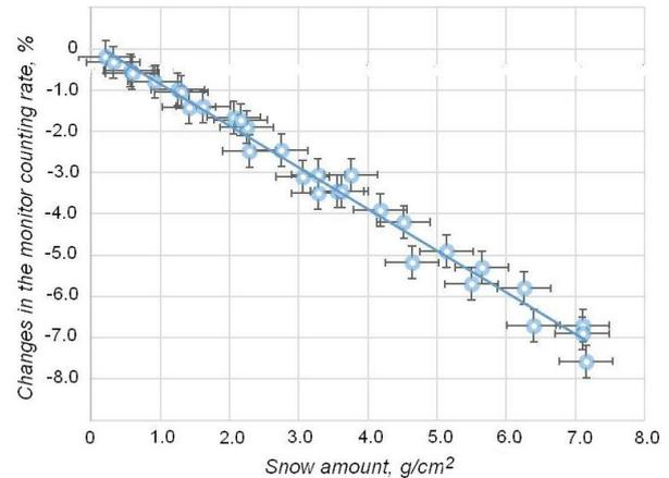
Figure 4. Count rate of the neutron monitor versus the amount of snow above it
