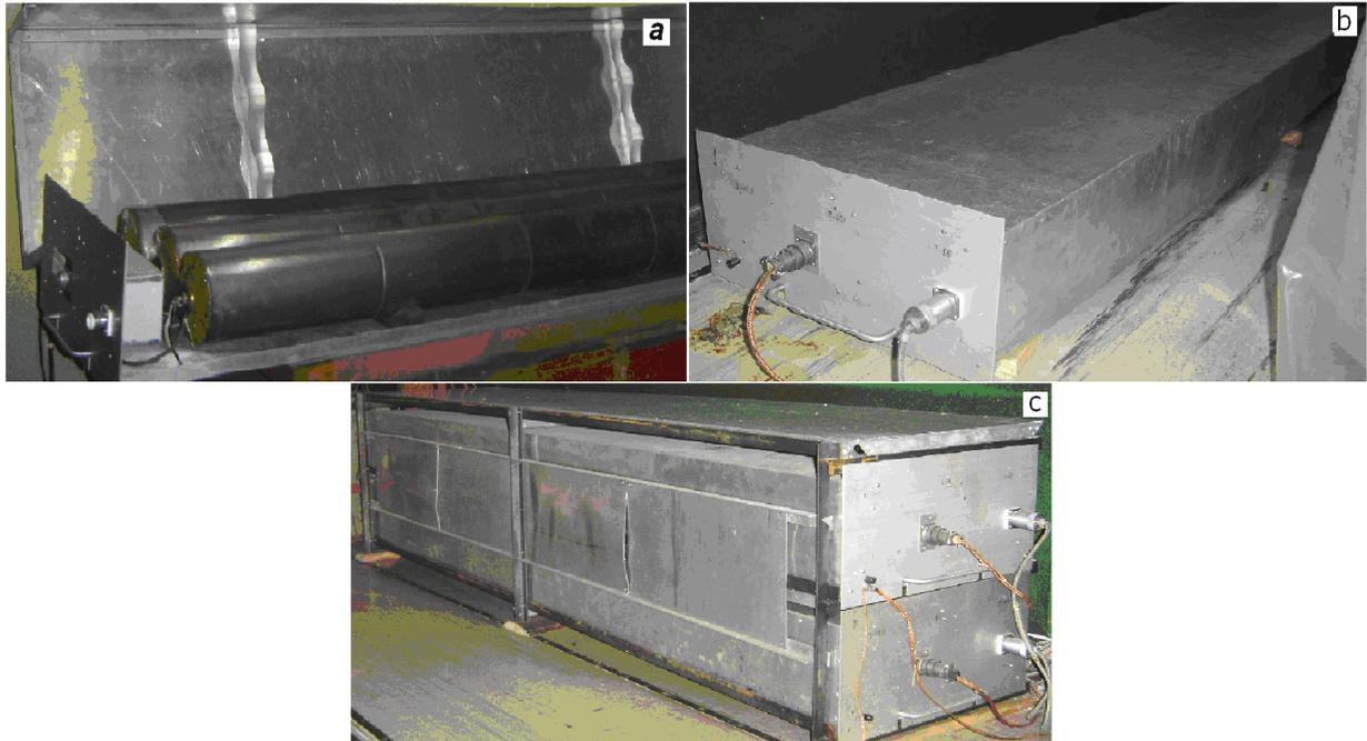
Figure 1. Neutron detector: arrangement of counters in a unit (*a*); a single remote detector unit (*b*); paired detector units (*c*)
