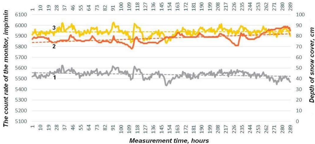
Figure 7. An example of a continuous synchronous recording of the neutron monitor count rate (curve 1) and snow depth on the roof of a building (curve 2). The monitor count rate corrected for the effect of snow is shown by curve 3. Dashed lines indicate monitor count rate trends (initial data), snow depth over the measurement period, and the monitor count rate corrected for the effect of snow.
