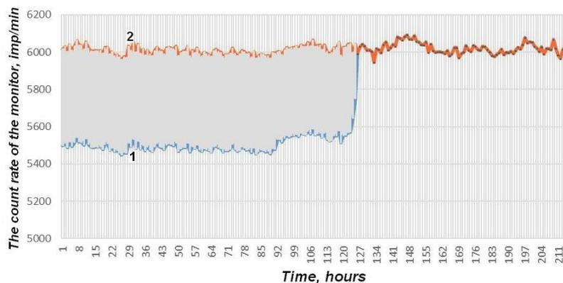
Figure 8. Change in the neutron monitor count rate when the accumulated snow melts from the roof of the building
