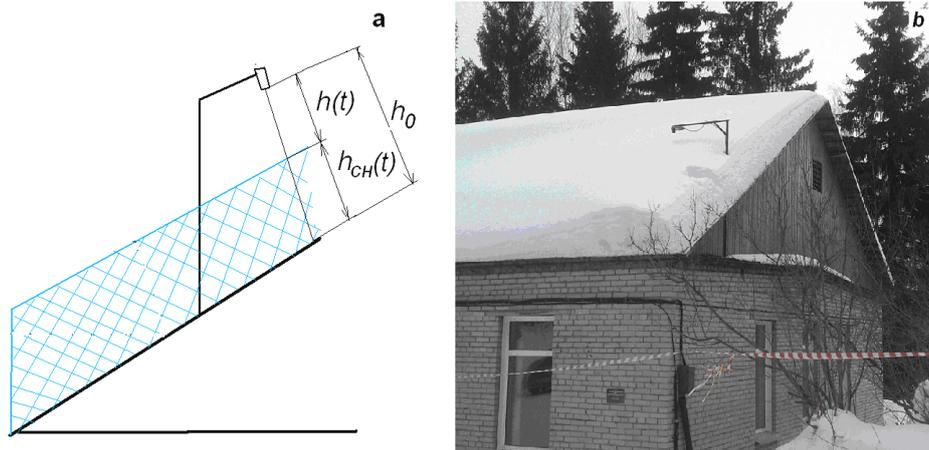
Figure 6. Installation of a snow gauge sensor above a building: scheme (a) and general layout (b)
