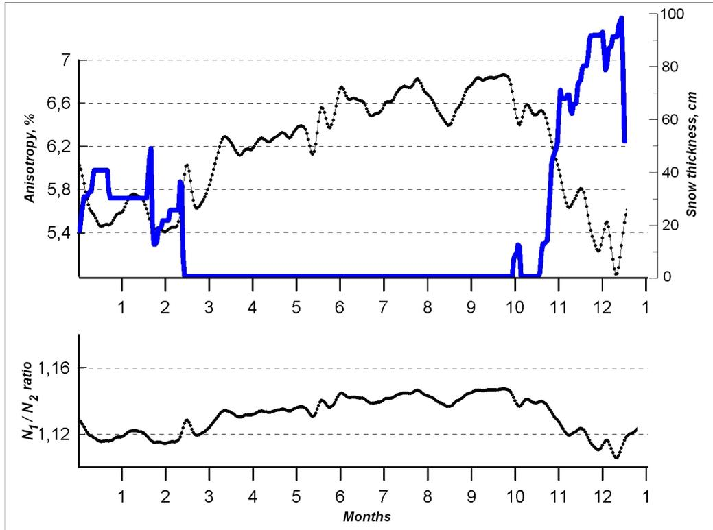
Figure 2. Seasonal variations in the thermal neutron flux near Earth's surface: at the top — flux anisotropy (black curve) and snow depth (blue curve); at the bottom — a ratio between count rates of detectors  $N_1$  and  $N_2$
